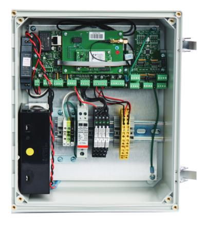
The HTT GEN-2 offers a significant evolution over High Tide Technologies' legacy series of RTUs. While the capabilities of the previous series were impressive, this next-generation RTU raises the bar even higher with faster data poll readings, a fully functional Modbus interface, over-the-air firmware updates, and more.
