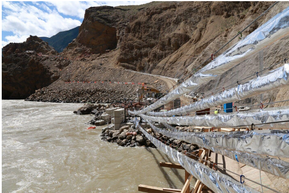
Figure 9. Six-Lane Pneumatic Fish Transport Tube System (Whooshh) at the Big Bar Emergency Fish Transport Site, Fraser River, British Columbia.
