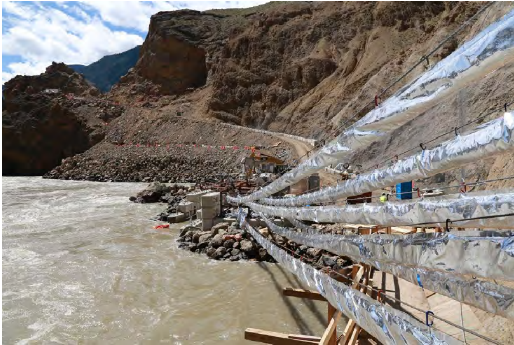
Figure 9. Six-Lane Pneumatic Fish Transport Tube System (Whooshh) at the Big Bar Emergency Fish Transport Site, Frasier River, British Columbia.
