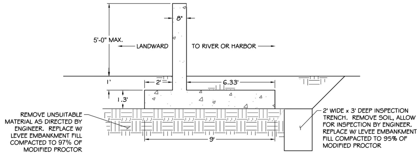
○ TYPICAL CONCRETE FLOOD WALL SECTION
